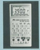
**DESCRIPTION:** A programmable, autoranging 33/4-digit DMM with an analog bargraph display, a dBm function for audio/communications, and 0.25% basic DCV accuracy. An upgrade of the AR-3100, this meter is water and contaminant proof
