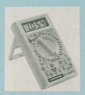
DIGITS: 31/2 DC VOLTAGE RANGE: 1000 volts, 5 ranges **AC VOLTAGE RANGE: 750**
