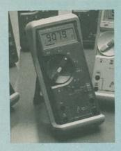
and a smoothing function that displays a running average of last 8 readings.
