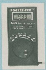
DIGITS: 31/2 DC VOLTAGE RANGE: 500 volts, 5 ranges AC VOLTAGE RANGE: 500 volts, 4 ranges CURRENT RANGE: N.A. **RESISTANCE RANGE: 20** megohms, 6 ranges SPECIAL FEATURES: Autoranging, data hold, diode test, audible continuity test, data hold. auto polarity, built-in test probes, carrying case DIMENSIONS/WEIGHT: 4.4 ×
