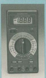
DMM with transistor gain and capacitance measurement features.
