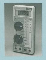
ranges AC/DC **RESISTANCE RANGE: 20** megohms, 5 ranges SPECIAL FEATURES: Diode test, audible continuity test DIMENSIONS/WEIGHT: 7.1 × 3.4 × 1.8 inches/1 pound PRICE: \$200.00
